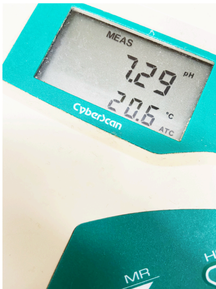
Figure 2.2: The digital display of a pH meter. Since pH is calculated using a logarithmic function, the value displayed has only 2 significant figures. Photo by Julian Pakay.
