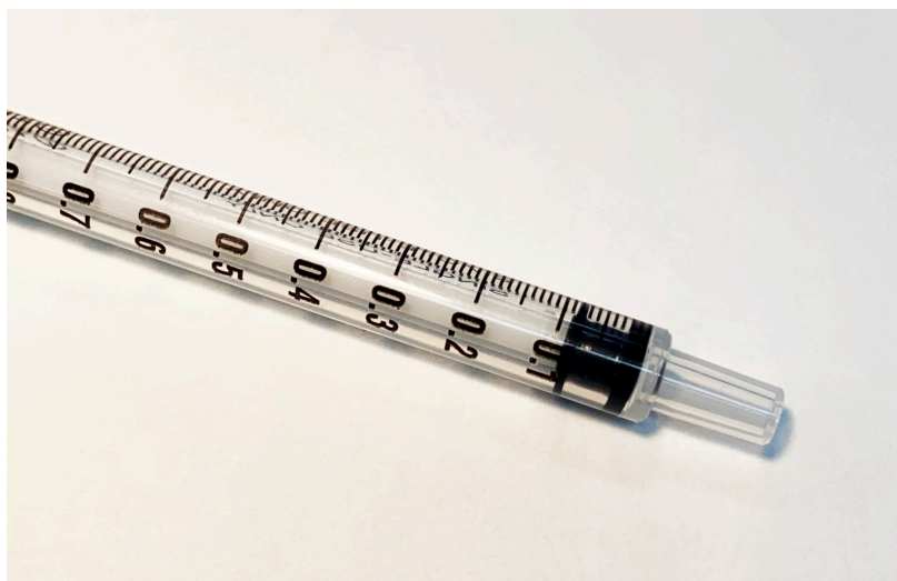
Figure 2.1: A 1 ml Luer lock syringe showing 0.1 ml major increment markings each divided into 0.01 ml gradations.
